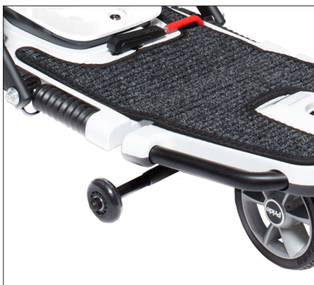
Front Stabilizing Wheels for Safety
